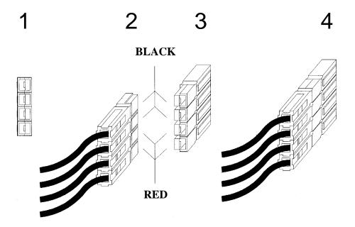
Caution: Make sure the UPS is shutdown and unplugged before connecting additional Battery Packs (refer to Switching the UPS "Off" section, page 11)
